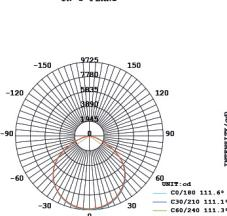
INTENSITY DISTRIBUTION DIAGRAM IN C PLANS
