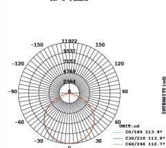
INTENSITY DISTRIBUTION DIAGRAM IN C PLANS
