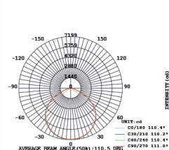
INTENSITY DISTRIBUTION DIAGRAM IN C PLANS
