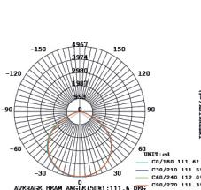
INTENSITY DISTRIBUTION DIAGRAM IN C PLANS
