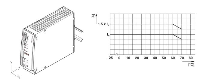
Rotated mounting position 90° X-axis
