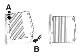
Figure 6 Assembly on standard DIN rail
