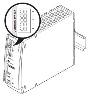
Figure 13 Position of output terminals
