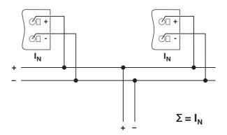
Figure 21 Schematic diagram in parallel operation
