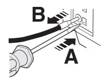
Figure 9 Release connecting cable (push-in connection technology)
