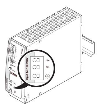
Figure 11 Position of input terminals
