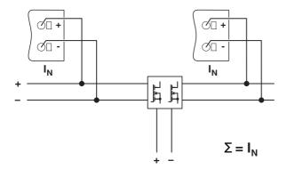
Figure 23 Schematic diagram, decoupling with ORING module
