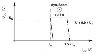
Figure 15 U/I characteristic curve with dynamic load reserve
