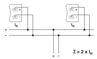
Figure 24 Schematic diagram of increased performance
