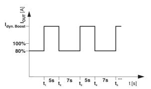
Figure 16 Schematic diagram of dynamic boost behavior
