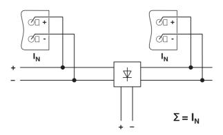
Figure 22 Schematic diagram, decoupling with diode module
