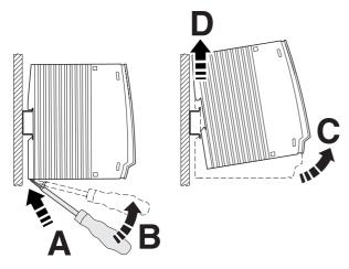
Figure 7 Removing the DIN rail
