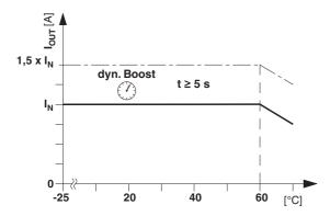
Figure 19 Temperature derating in normal mounting position
