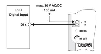
Figure 18 Wiring principle
