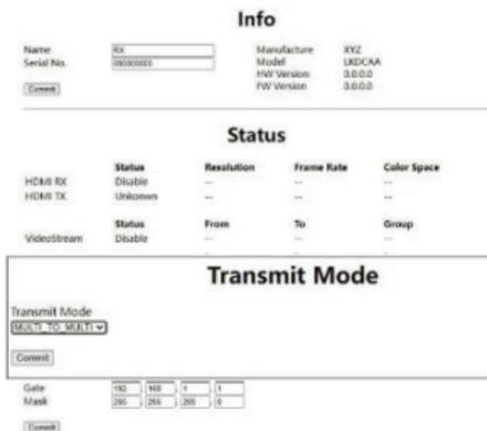
As a maximum of 8 transmitters can be connected, the IP addresses of each of them must be assigned in ascending order in the “Ethernet” section. Simply change the last number of the address.
