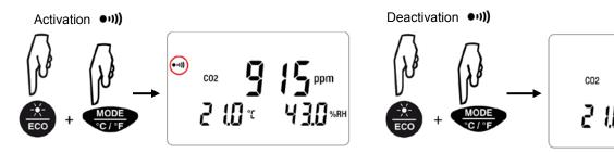
First press the **ECO** key, then, while keeping it pressed, press the **MODE** key.
