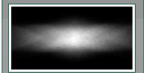
Beam Type: Elliptical Beam Angle: 140 x 60 x 0
