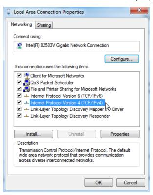
Step 9 Select Use the following IP address, set the IP address to 192.168.2.X (X ranges from 2 to 253), the Subnet mask to 255.255.255.0, and click OK.
