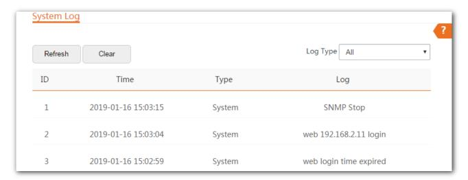
To ensure that the logs are recorded correctly, verify the system time of the device. You can correct the system time of the device by choosing **Tools** > **Date & Time**.
