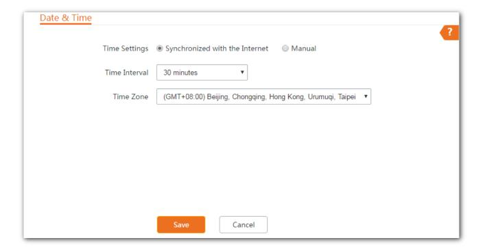
The device allows you to set the system time by synchronizing the time with the internet or manually setting the time. By default, it is configured to synchronize the system time with the internet.
