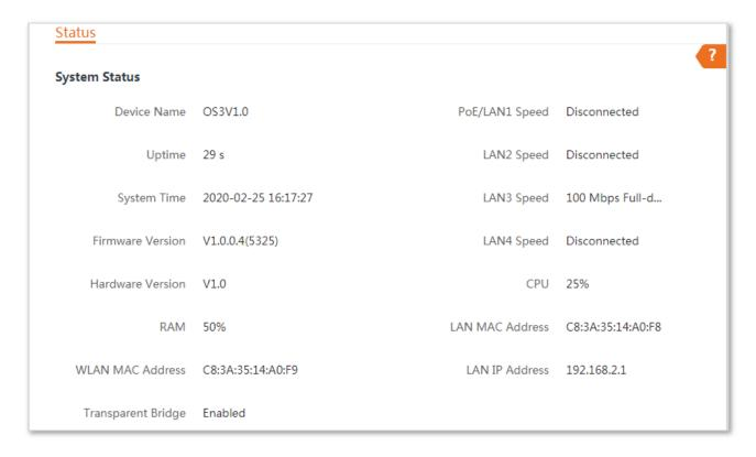
If the device is set to **WISP** or **Router** mode, the system status is shown as follows:
