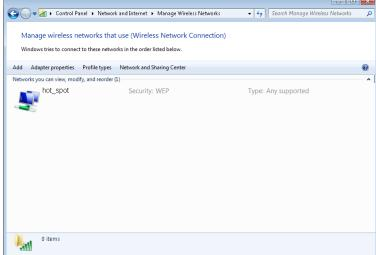
**Step 12** Click the network icon in the lower-right corner of the desktop and choose the wireless network of the CPE such as **hot\_spot** in this example.
