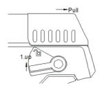
Lift the side trigger upwards and pull the rear block backwards: this will cause the release of the accumulation channel.
