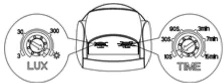
*Note: when testing in daylight, please turn LUX knob ☀ (SUN) position, otherwise the sensor lamp could not work!*
