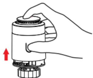
Gently pull up the housing cover while pressing down on the rotary plate with the index finger
