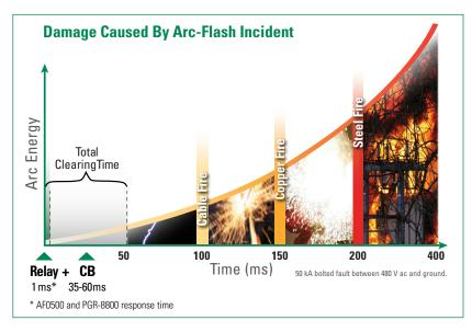
The Littelfuse Arc-Flash Relays use a 125-µs light-sampling scheme in combination with an ultra-fast IGBT output to be able to detect a developing arc flash and send a trip signal to a circuit breaker in milliseconds.
